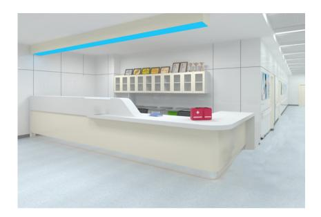
The table top is made of 25 mm thick high density fiberboard (HDF) and is finished with 12 mm thick corian solid surface.
